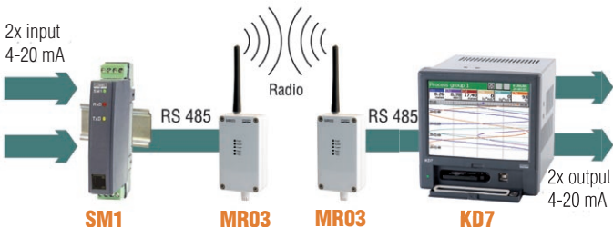
Fig 1. Example of remote readout of data between KD7 recorder and analog input module, type SM1 using MR03.
